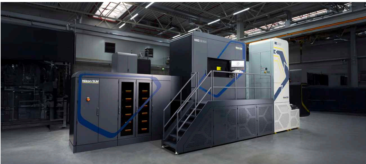
NXG XII 600® with RELOOP automated powder management system.
