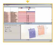
The geometrically similar part that was found can then be compared and measured with the constructed part in a 3D view.
